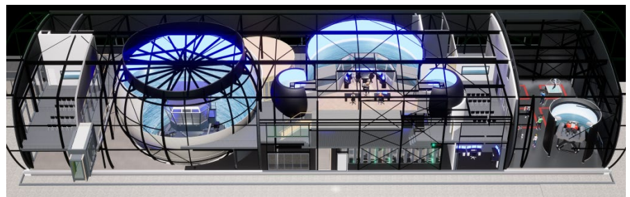
The Large Motion Simulator (on the left) in the SOSc with a moving bridge of 4 x 5 m on a hexapod and the Full Mission Bridge Simulator (in the middle).
